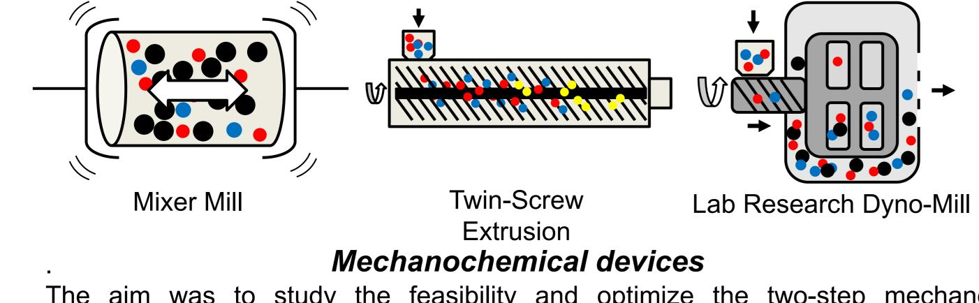
The aim was to study the feasibility and optimize the two-step mechanochemical Beckmann rearrangement starting from acetophenone and 4-hydroxyacetophenone to form acetanilide and paracetamol, respectively, with the Dyno-Mill.
